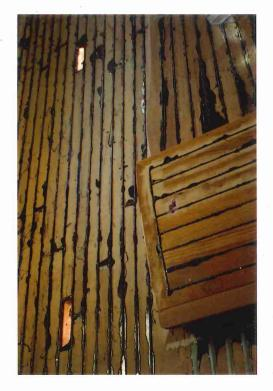
The ship is not caulked. Not a single nail or screw is used. All parts are connected by wooden pins, ultra modern adhesives and saturated with epoxy. Because of the seamless construction of the planking, impermeability to water and stifness of the hull is well improved.
